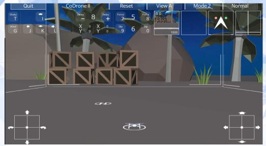
(5) Hold the L1 button for more than 1 second to take off/land and control the drone with the controller.
