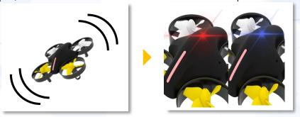
When the drone is ready for pairing, the LED on the top of the drone is red and blue.
